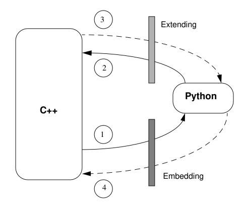
In this picture, C++ and Python are depicted as separate systems; in reality, Python is bound-in to the C++ process/executable, so the distinction is only a logical one [more dynamic communication structures are possible, but not planned]. Some notation:
